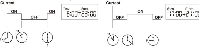
NOTE: If the main power is turned OFF or a power failure occurs while ON/OFF timer is active, the timer setting is cancelled. As these models are equipped with an auto restart function, the air conditioner starts operating with timer cancelled when power is restored.
